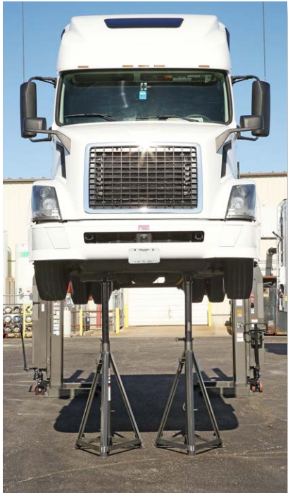
Model 9-THR High-Rise vehicle support stands working with Gray's Patented Wireless Portable Lift System
