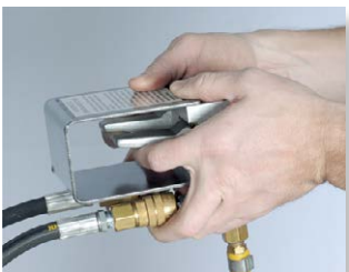
Dual trigger control valve allows synchronized raising and lowering of vehicle.
